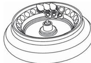
**!** *To avoid potential breakage of the microcentrifuge tube cap during centrifugation, insert the purification column/ 0.5 mL tube assembly into a lidless 1.7/2.0 mL tube. Insert this assembly into adjacent rotor holes as illustrated. Rest the tube cap against the tube immediately clockwise to it. Place an empty, lidless 1.7/2.0 mL tube into the rotor hole adjacent in the clockwise direction to the last assembly.*
