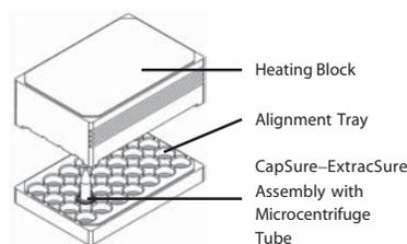
**!** The CapSure HS LCM Caps and the ExtracSure Device are compatible with 0.5 ml thin-walled reaction tubes from Applied BioSystems. These reaction tubes should be used for RNA extraction.
