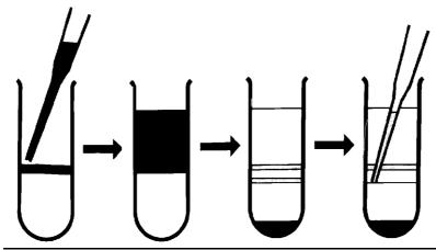
Isolation of polymorphonuclear granulocytes using Lympholyte®-poly. After centrifugation, the upper monolayer is mononuclear cells, and the bottom monolayer is polymorphonuclear cells. Erythrocytes and dead cells are found in the pellet.
