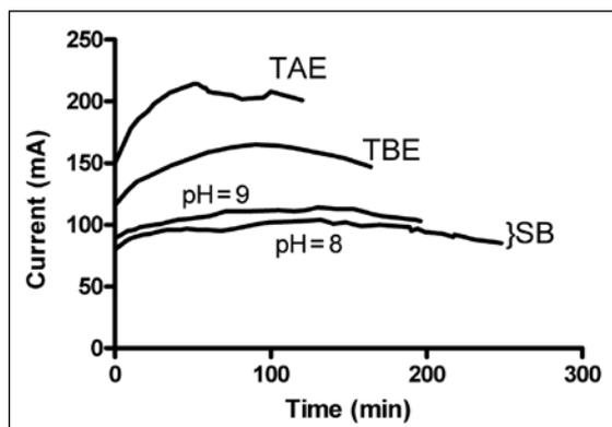
**Figure 2. Electrolyte exhaustion.** Conductive media were tested by plotting the current at constant voltage (200 V). TAE, Tris-acetic acid-disodium EDTA; TBE, Tris-boric acid-disodium EDTA; SB, sodium boric acid.
