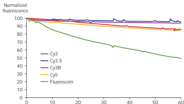
Fig 24. Photostability of fluorophores under "natural" light conditions.
