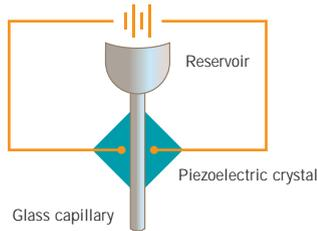
Fig 10. Diagram of a piezoelectric microarray printing system.
