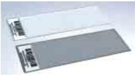
**Fig 4.** A glass microarray. A standard and mirrored glass microscope slide that contains several thousands of immobilized cDNA fragments. Because of the small amounts of nucleic acid present and their tiny size, the target spots are not visible with the naked eye.
