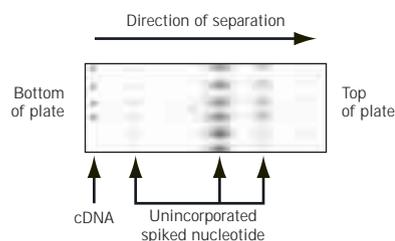
**Fig 51.** Thin layer chromatography analysis of the incorporation of radioactive spike into labelled cDNA sample. The labelled nucleic acid does not migrate far from the sample application line, whereas the unincorporated radioactive nucleotide moves up toward the top of the plate.
