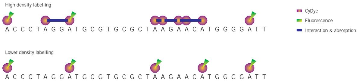
**Fig 32.** Quenching and labelling density. Fluorescent output from two identical nucleic acid strands labelled to different labelling densities is depicted. Green denotes fluorescent emission whereas purple shows energy being lost in intermolecular interactions between adjacent fluorophores. Lower labelling density results in higher fluorescent signal.
