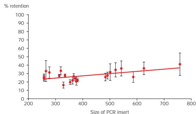
Fig 8. Retention of microarray targets of different lengths on aminosilane-treated microarray slide.
