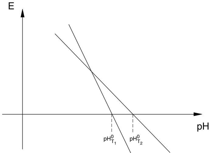
*Fig. 2. The mV/pH relation at two different temperatures*
