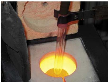
*The base of the electrode is dipped into an oven of molten glass at a temperature of 1200 °C.*
