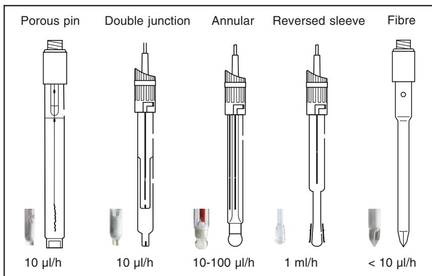
Fig. 5. Liquid junction constructions with typical KCl outflow
