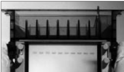
Fig 2.8. Locking the upper buffer chamber in place.
