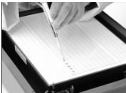
Fig 3.6b. Pipetting samples into the applicator strip wells.
