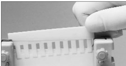
Fig 2.14. Remove comb and wash wells to remove unreacted acrylamide.
