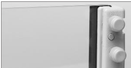
Fig 2.2c. Properly assembled gel sandwich. Glass plates and spacer are flush.
