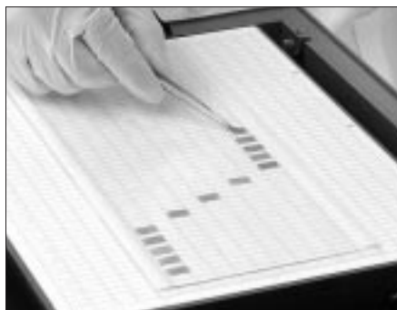
Fig 3.12. Placing sample application pieces across the gel.
