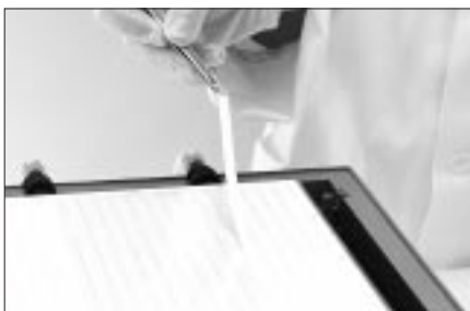
Fig 3.5. Applying an electrode strip near the anode.
