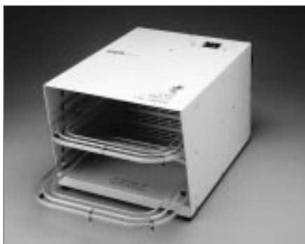
Fig 4.5 Hoefer SE 1200 Easy Breeze Air Gel Dryer.
