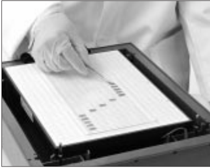
Fig 3.9a. Placing sample application pieces across the gel.
