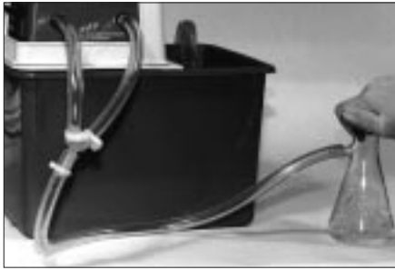
Fig 2.3. Mixing the gel solution under vacuum (step 3). A water aspirator is a convenient choice for this procedure.
