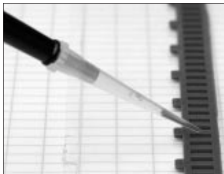
Fig 3.13. Pipetting samples into applicator strip wells.
